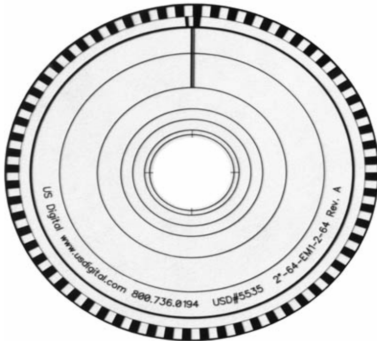
Figure 3.10. Patterned line disk which rotate in the shaft between an LED and detector to produce square waves for digitization seen in Figure 3.11.
