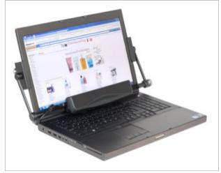
Figure 51. The Tobii X1 Light Eye Tracker allows the researcher to conduct eye-tracking studies in the field using a laptop.
