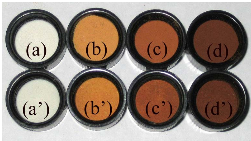
Figure 6.5 Different colors of various samples. (a) as-synthesized Ti-a nanotubes, (a') as-synthesized Ti-w nanotubes, (b) MEHQ-Ti-a-70°C, (b') MEHQ-Ti-w-70°C, (c) HQ-Ti-a-70°C, (c') HQ-Ti-w-70°C, (d) CAT-Ti-a-70°C, (d') CAT-Ti-w-70°C.
