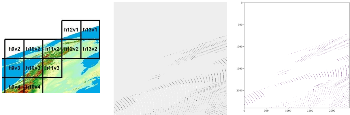
Figure 14. MODSCAG tile h10v02, representing Alaska, for January 1 st , 2004. (A) shows the geographic extent of the MODSCAG tiles, with h10v02 shown on the second row (map produced by Karl Rittger), (B) is the raw tif file, and (C) is the processed tile, with any SCF values between 0-100 shown.
