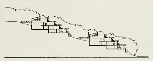
Housing development appropriate to a mid-slope site to cated on an inner suburban hillside. Density has been kept tow by clustering the units, leaving much of the forested hillside untouched.
