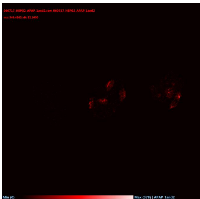
Appendix chapter 5 figure 8 MSI of small molecule species ( m/z=549.4863 ) present within the hydrogel at cell locations.
