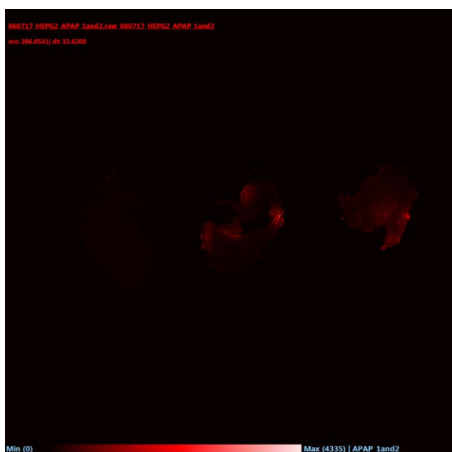
Appendix chapter 5 figure 5 MSI of small molecule species ( m/z=206.0541 ) present within the hydrogel at cell locations.
