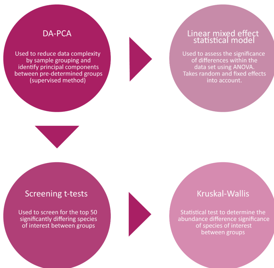
Figure 3.2 Workflow diagram of the statistical tests used to determine significantly different ionic species.
