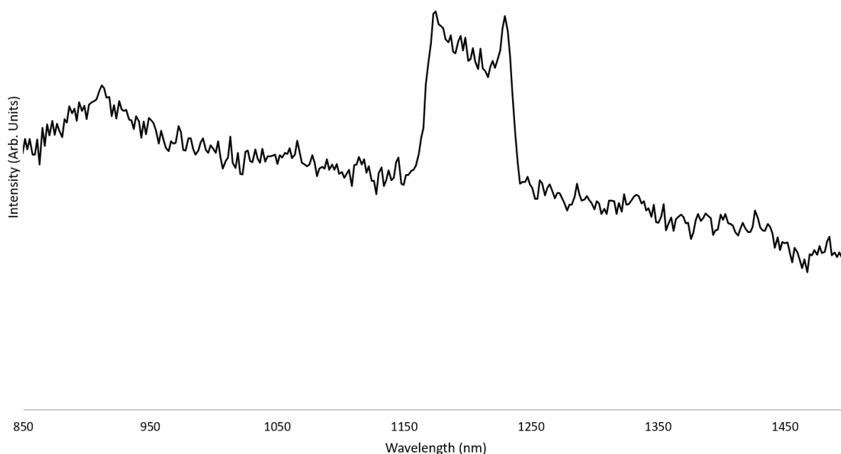
Figure 88 NIR fluorescence emission spectra of 0.20mol% \text{Bi}_2\text{O}_3 SLS (ex 12,500 \text{ cm}^{-1} 800 nm)
