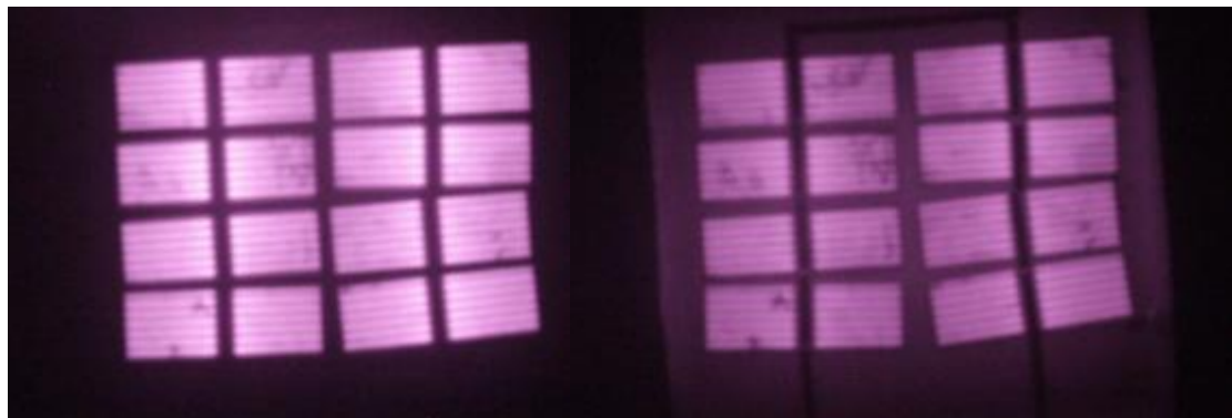
Figure 102 Electroluminescence of string (left) and module (right) float glass PV module
