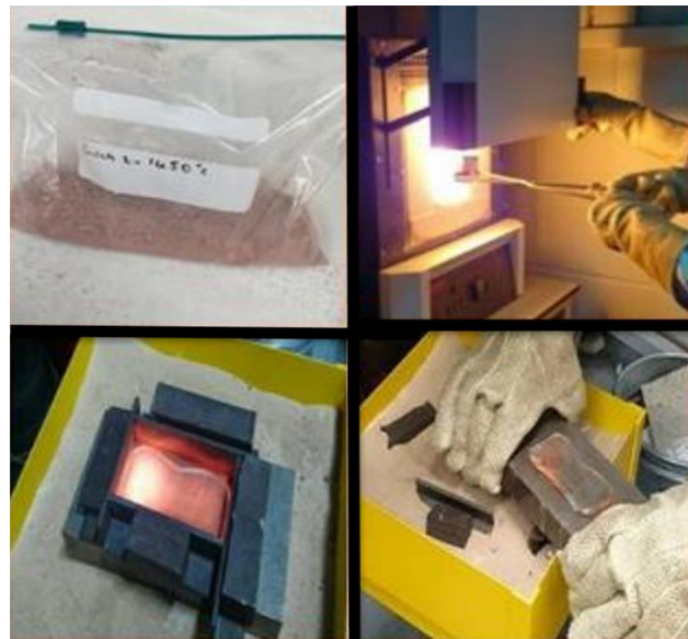
Figure 39 Melt quench process for the lab scale production of SLS glasses
