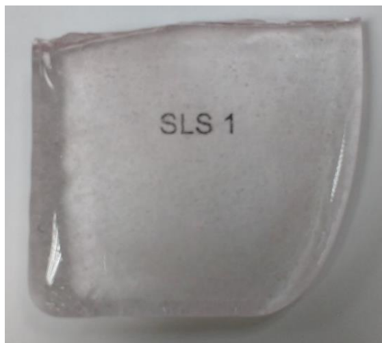
Figure 35 SLS1, pink discoloration and bubbles
