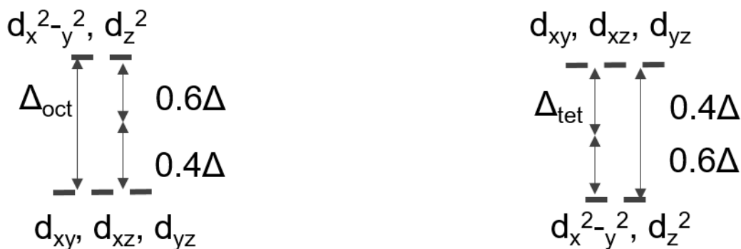
Figure 33 Splitting of d-orbitals due to octahedral ligand field (left) and tetrahedral ligand field (right)
