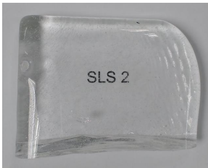
Figure 37 SLS2, no pink hue, with bubbles remaining
