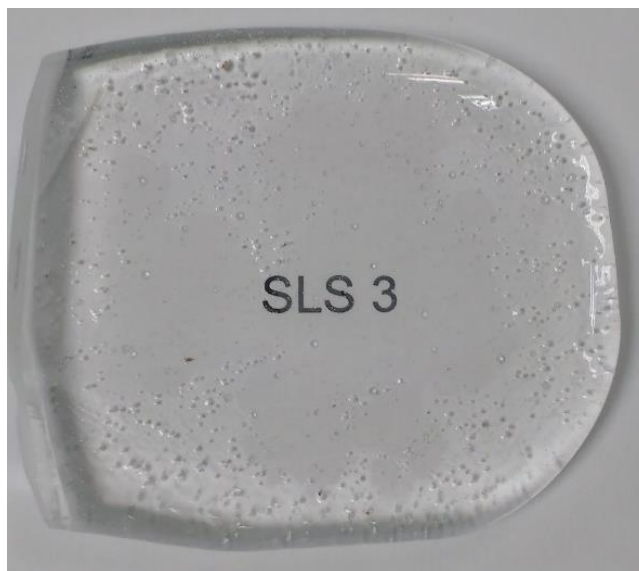
Figure 38 SLS3, with bubbles remaining
