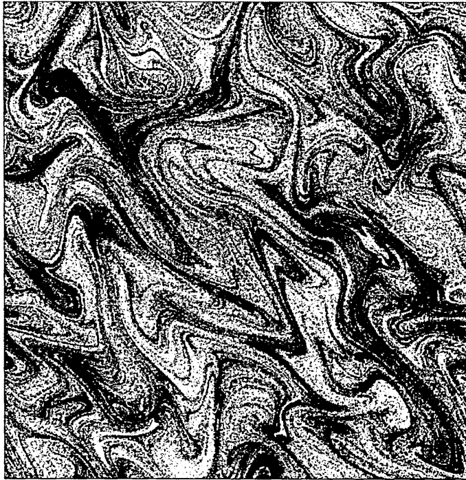
Figure 3.1: Distribution of particles with significant inertia moving in a two-dimensional incompressible velocity field (the equations of motion are specified in section 3.2). The particles tend to cluster and for the parameters used in this simulation (see section 3) the correlation dimension is D_2 \approx 1.76
