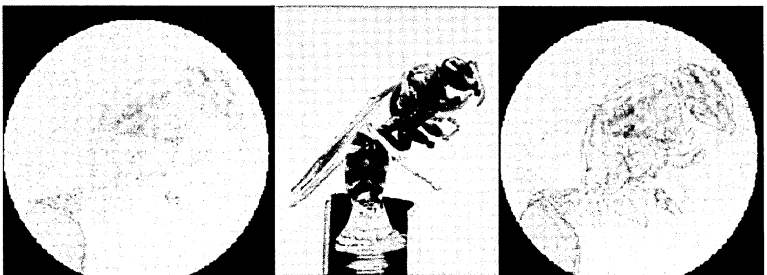
Figure 2.3.10: Comparison between standard neutron radiography and phase contrast radiography [80] of a yellow jacket wasp. A higher clarity for finest features (e.g. antenna, legs) is revealed through phase contrast imaging.
