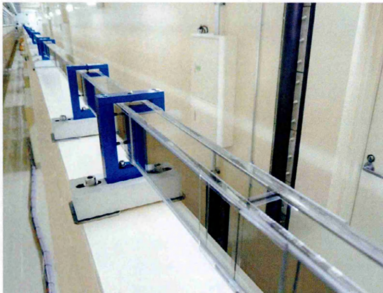
Figure 3.4.3: Straight rectangular neutron guide section coated with supermirrors ( m=3 ) for J-Parc fabricated by SwissNeutronics [152].
