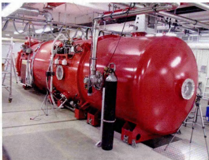
Figure 6-1: Image of the Mars Simulation Wind Tunnel Facility.
