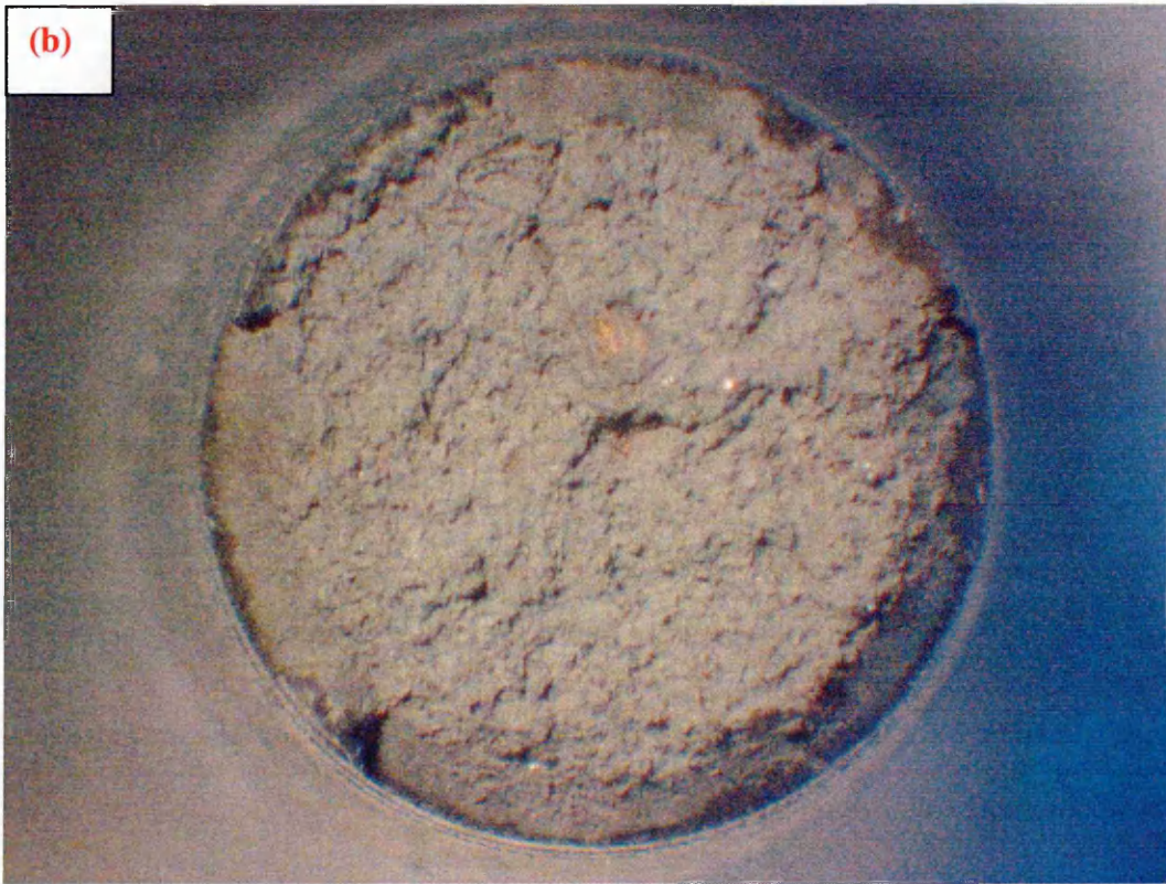
Fig. 5.12 Macro images showing gold coloured inclusions on fracture surface of different 410L MA samples from the second batch
