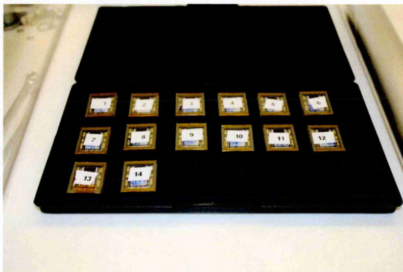
Figure 8-9. Fourteen CCD97s ready for testing at the HIF in Louvain.
