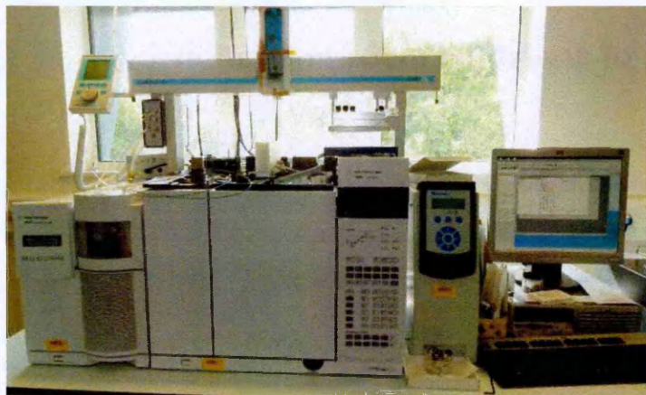
Figure A.6: An Agilent 7890 N interfaced with a 5975 quadrupole mass spectrometer and a CTC CombiPal autosampler that was utilised for the analysis of HAAs in electron capture negative ionisation.
