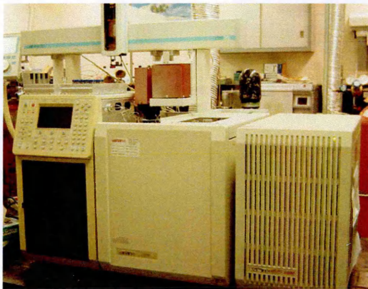
Figure A.4: A Varian CP-3800 gas chromatograph interfaced with a Saturn-2000 ion trap mass spectrometer, and a CTC Combi Pal autosampler were used for the analysis of THMs.
