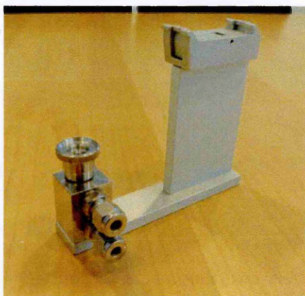
Figure A.10: A flow-through cell which can be interfaced on a CTC CombiPal autosampler system for the possible near-real time analysis of THMs.
