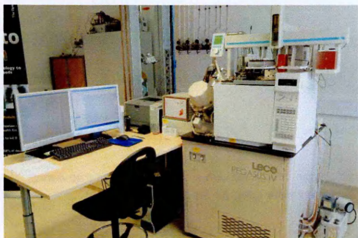
Figure A.7: Agilent 6890 N gas chromatograph fitted with a GCxGC cryogenic modulator coupled to a Leco Pegasus IV time-of-flight mass spectrometer and a CTC CombiPal autosampler (GCxGC-ToFMS) used for the analysis of HAAs.
