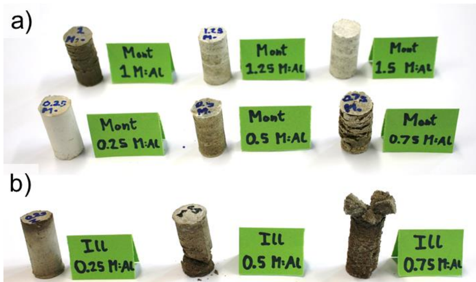
Figure 5-12: Photos of the cured samples of a) montmorillonite series and b) illite series. Samples were cured in 18 mm diameter, 36 mm height cylindrical moulds.
