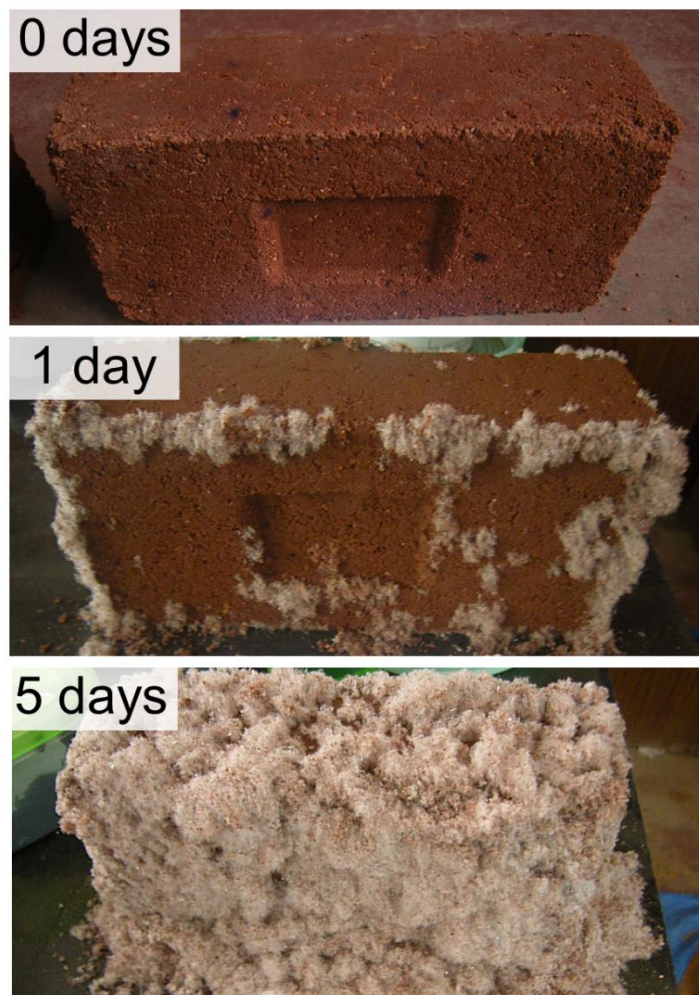
Figure 8-9: The act-0h block specimen after demoulding (0 days), and after 1 and 5 days ageing.
