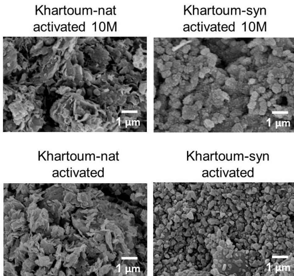
Figure 7-19: SEM images of the 10 M and original 4.1 M activated samples of the natural and synthetic Khartoum soils.
