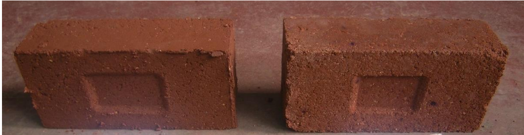
Figure 8-8: Comparison of the control (left) and activated (right) block specimens immediately after compaction and demoulding.
