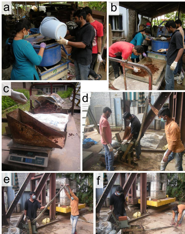
Figure 8-2: Stages in block specimen manufacture: a) mixing the soil, sand and activating solution, b) breaking up any remnant lumps in the wet mix, c) weighing out a set amount of wet mix for each block specimen, d) filling the mould with the wet mix, e) compacting the block specimen, f) releasing the block specimen from the mould.
