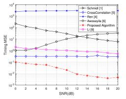
Fig. 4. Timing MSE of different algorithms in the COST 207 RA Channel.
