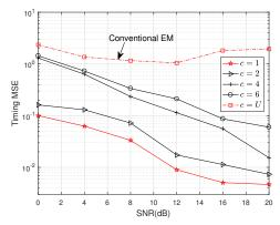
Fig. 2. Timing performance for different values of c for COST 207 RA channel.
