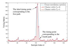
Fig. 1. Timing metric and classification results for COST 207 RA channel.
