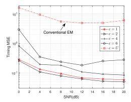
Fig. 3. Timing performance for different values of c for COST 207 TU channel.
