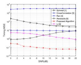
Fig. 5. Timing MSE of different algorithms in the COST 207 TU channel.
