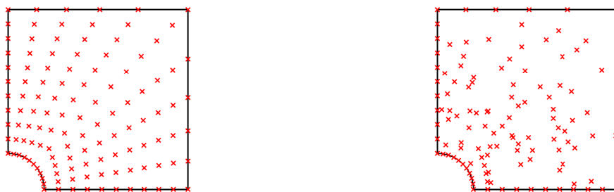
(a) A portion of the infinite plate with a circular hole with a far field stress p = 1.0 in x direction. (b) Collocation points after the 1st relocation.
