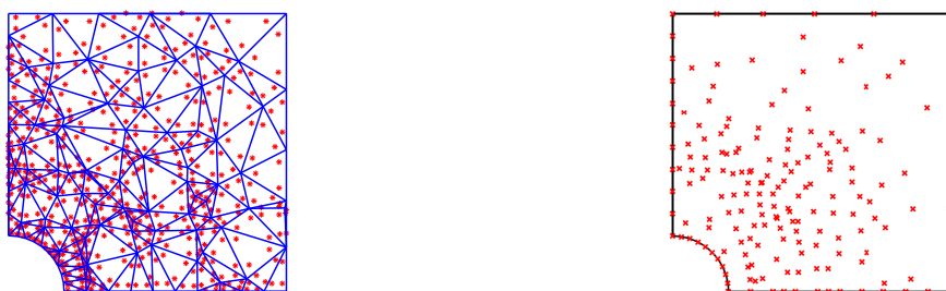
(c) The generation of triangles and calculation points. (d) Collocation points after the 1st rh -adaptivity.
