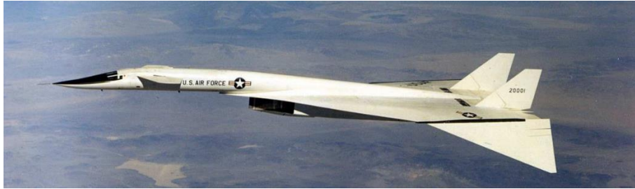
Figure 3. The XB-70 AV-1 in flight, with wingtips folded 25° downward at low supersonic speeds.
