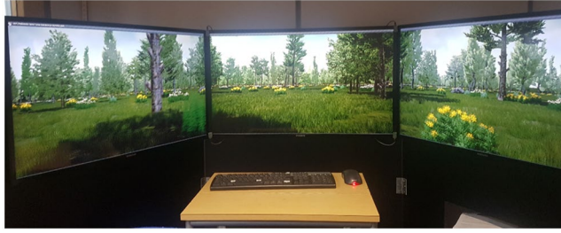
Figure 1. The 3-screen setup in the Bournemouth University Psychology Department. The two side screens are angled inwards at 60 degrees, giving a 180-degree horizontal field of view across all 3 screens.
