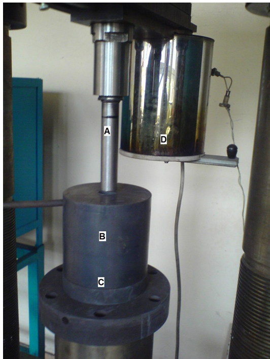
Fig. 2 Laboratory press (1000 kN) equipped with attachment for hot direct extrusion. By A the steel ram is marked, B is the container, C is the mounting position of extrusion die inside in container. By D electrical furnace for heating samples up to about 1100 °C is marked
