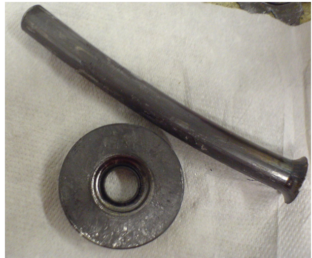
Fig. 3 Extrusion die and a rod after hot direct extrusion
