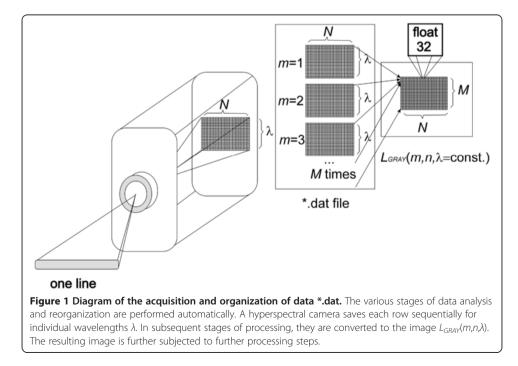
default bands, sensor type, interleave). For the analysed data, the image resolution  $M \times N$  was  $899 \times 1312$  pixels.
