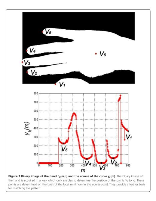
the centre of mass of the wrist calculated on the basis of the image  $L_O(m,n)$  resulting from the opening operation of the image  $L_B(m,n)$ , i.e.:
