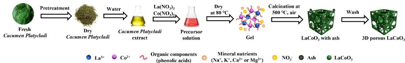
Scheme 1. Schematic illustration of the procedure to prepare bio-LaCoO 3 .
