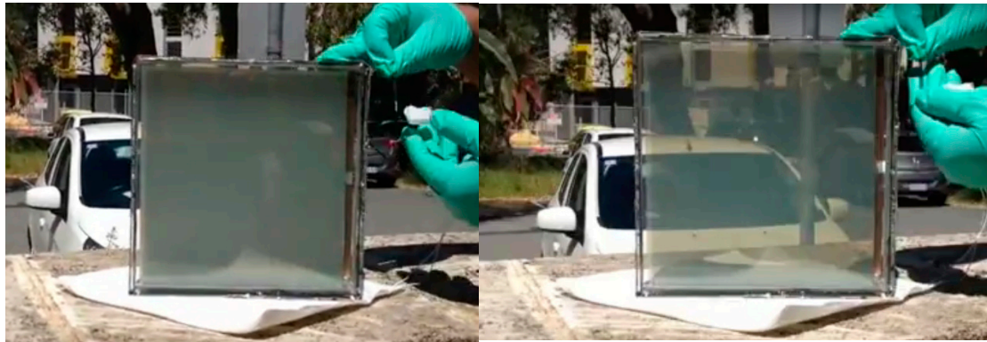
Figure 5. Transparency-controlled, self-powering PDLC-integrated “smart” solar window demonstration at Edith Cowan University (ECU) in October, 2014. A 200 mm × 200 mm hybrid concentrator-type solar window used four parallel-connected edge-mounted \text{CuInSe}_2 modules of size 198 mm × 25 mm, the electric output of which was sufficient to control the embedded PDLC layer transparency within a broad transparency range [108].
