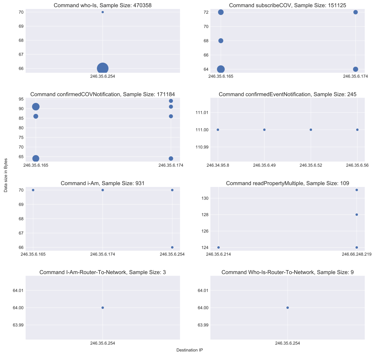
Figure 5.5: Scatter graph of packet size and destination for command packets sent by host 246.35.6.172
