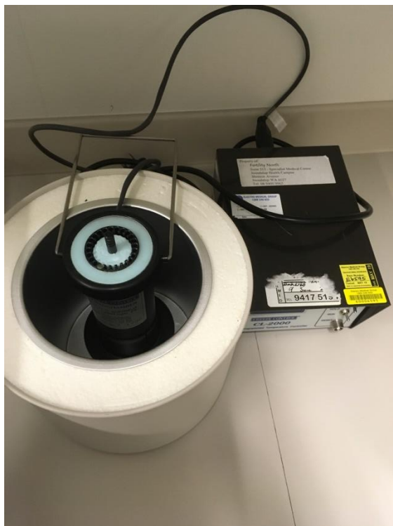
Figure 8. The CryoChamber within the CryoBath coupled to the CL-2000 freeze control system.
