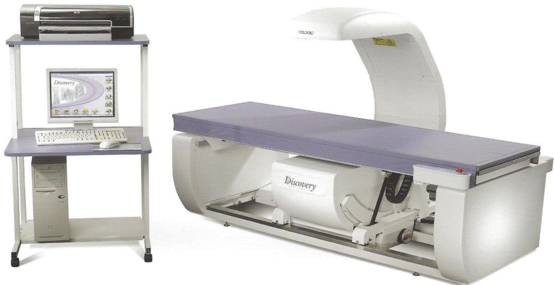
Figure 3. A fan-beam Hologic DXA (Discovery A) densitometry machine.
