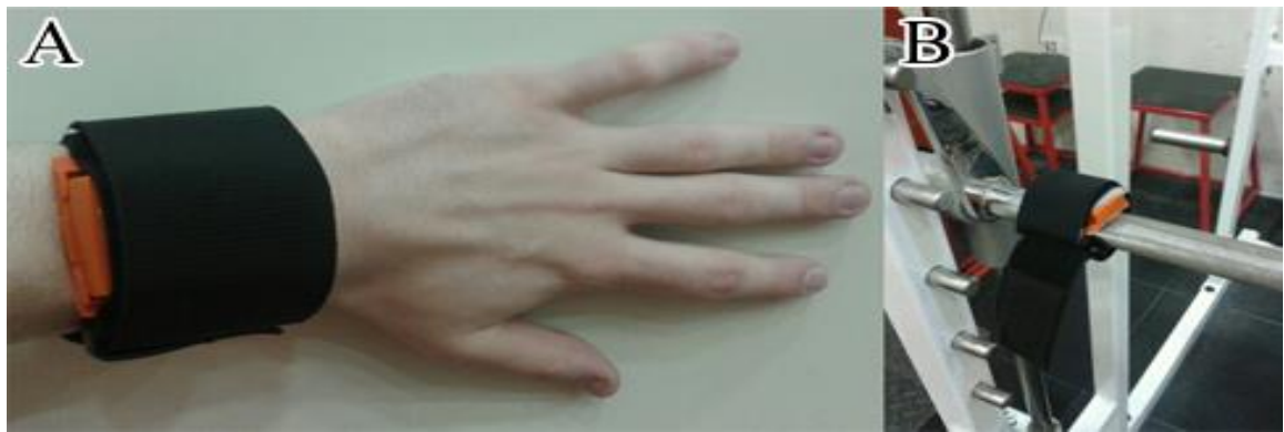
Figure 17. Positioning of the accelerometers on the wrist (A) and on the barbell (B).
