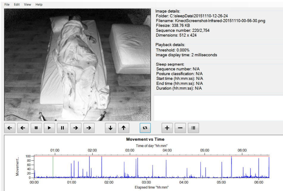
Fig. 1. Interface of the analysis software, showing a timeline and interactive movement graph at the bottom. The blue line on the chart indicates level of movement, the green vertical line corresponds to the current image being displayed and the red horizontal line represents a threshold for segmenting the session into different positions.
