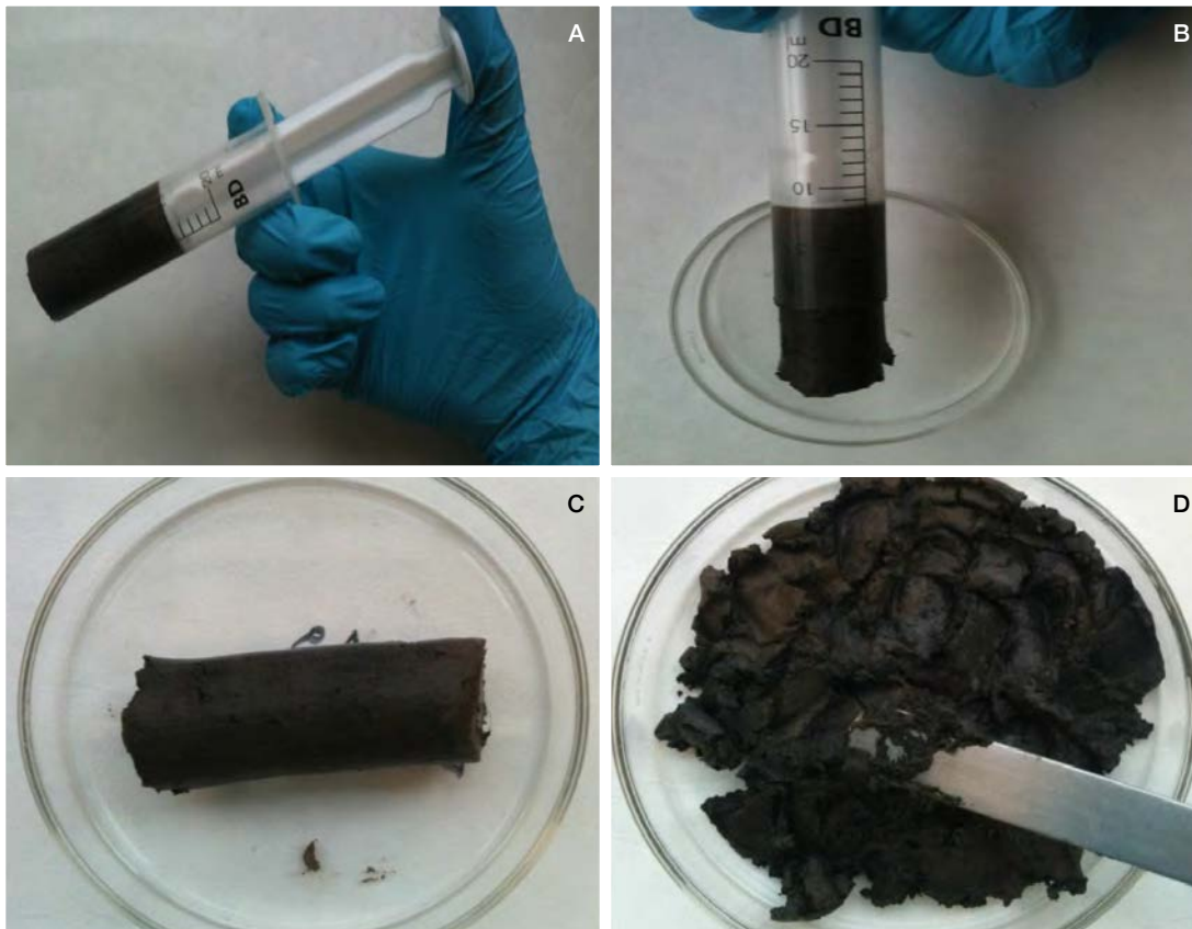
Figure 3.17 Removal of sample from syringe and preparing it for oven drying. (A) Sample in syringe, (B) Depositing sample on pre-weighed petri dish, (C) Sample when first removed from the syringe, and (D) Spreading the sample with a spatula. (© Hilary Kennedy, UWB)
