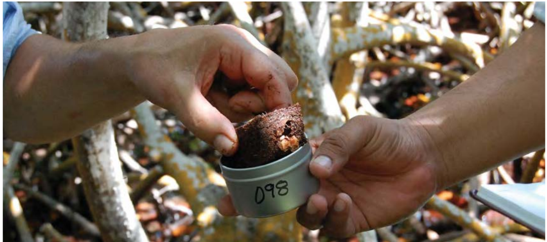
Figure 3.16 Samples are each placed in individual, numbered containers. The number corresponds with sample identification information recorded in the field notes. (© Boone Kauffman, OSU)
