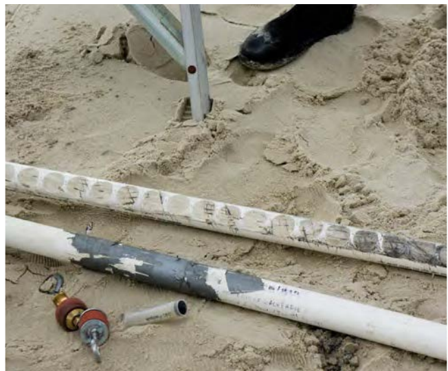
Figure 3.6 Seagrass coring devices. PVC tubes, rubber stopper, and syringe (© CI/Sarah Hoyt)
