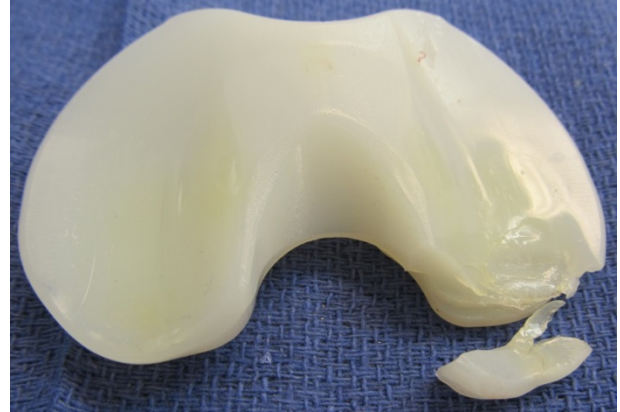
Figure 2. Polyethylene insert with significant posterior wear and posteromedial fracture.
