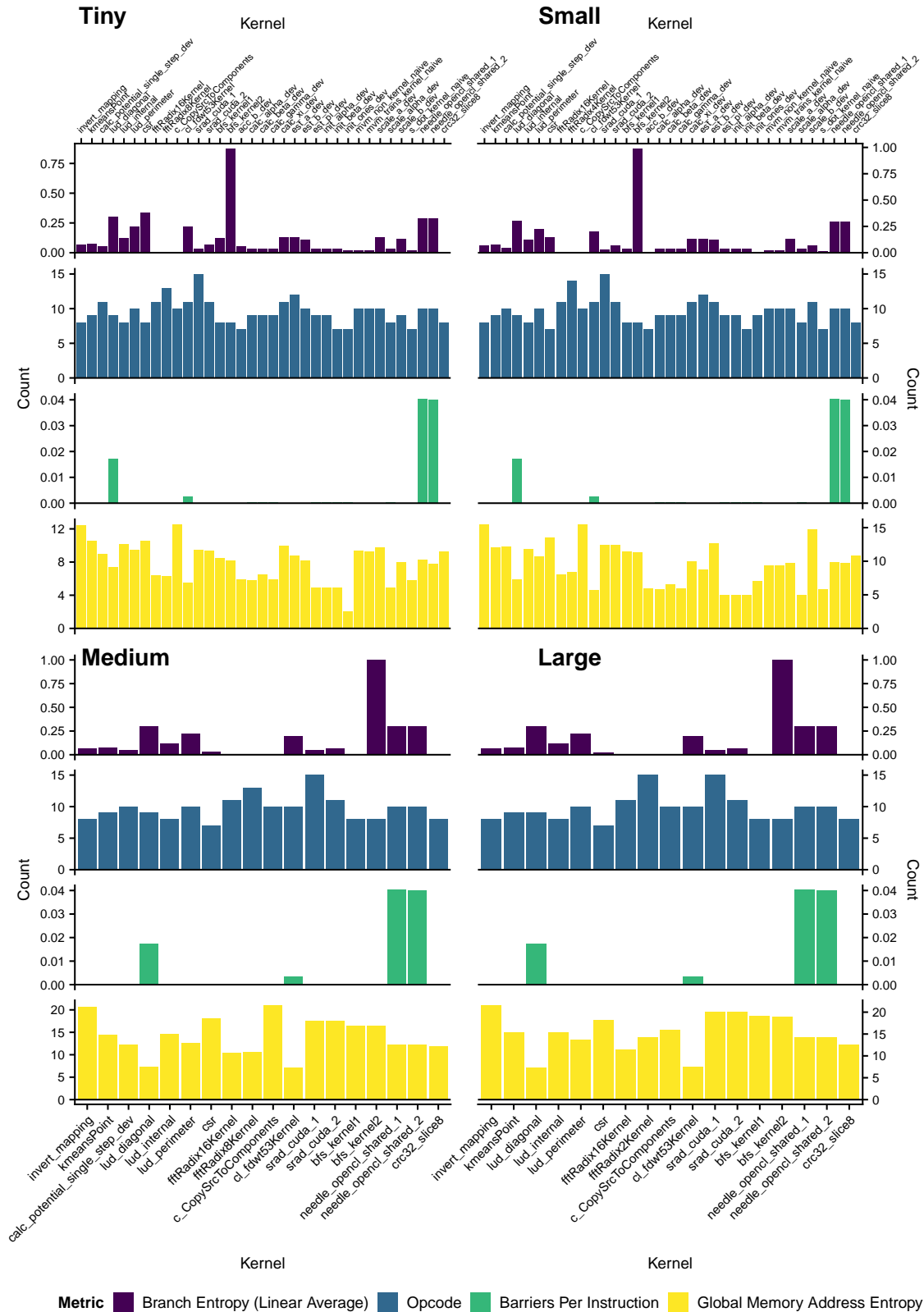
Figure 4.1: Selected AIWC metrics from each category over all kernels and 4 problem sizes.
