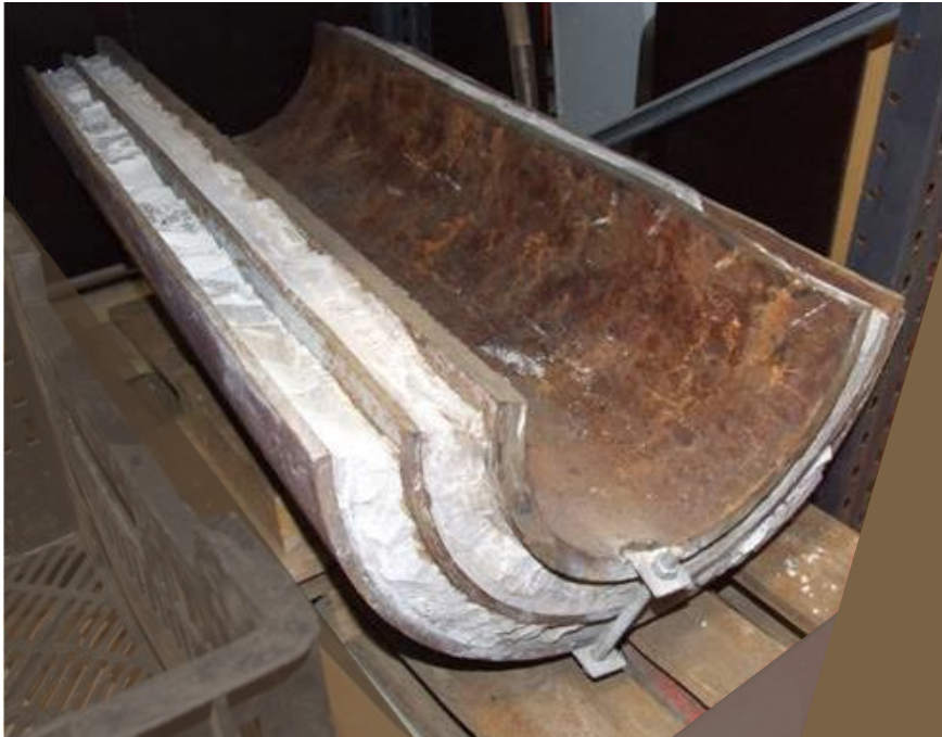
Figure 3.3: Cross-section of cemented casings that were excavated from a high-temperature geothermal well in Reykjanes, Iceland, showing the layered structure of casings and insulating cement sheaths (figure by Sigrún Nanna Karlsdóttir).
