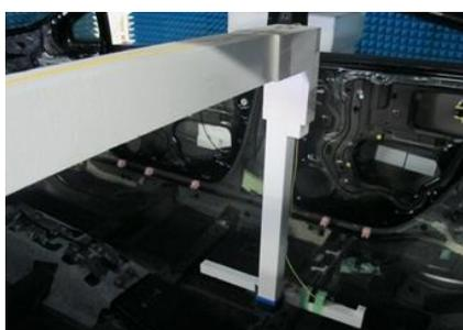
Measurement setup in vehicle cabin
