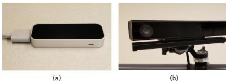
Figure 1: Devices used in V-HGR: (a) The Leap Motion controller, (b) The Microsoft Kinect 2
