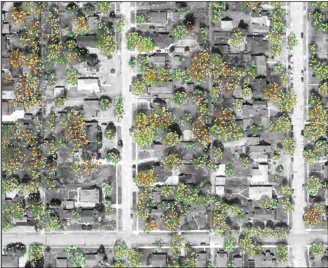
Figure 14. LiDAR Point Cloud After Filtering. Layered on top of a photograph of the area for visual confirmation of accuracy.
