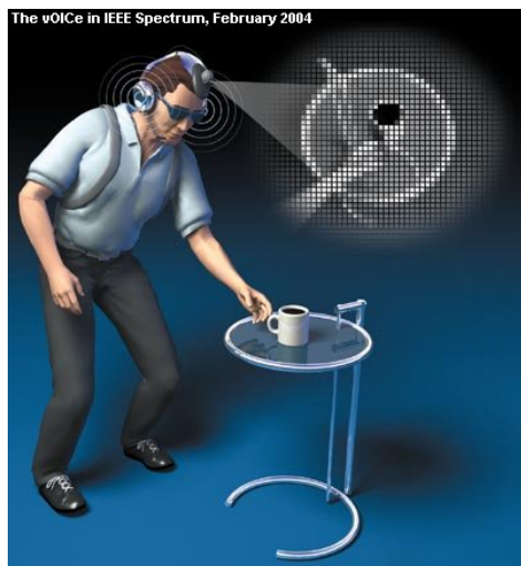
Figure 2: 3-D representation of the vOICe. A camera captures the scene and converts it into sounds through earphones (Jones, 2004).
