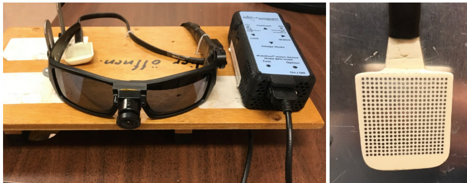
Figure 6: Image of the TDU. On the left are the glasses with a mounted camera, and right next to it is the BrainPort v100 remote. On the right is the 20x20 electrode array that subjects would place on their tongue.
