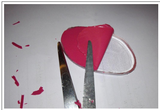
Fig. 3: Removing the pink cushion of silicone sponge.
