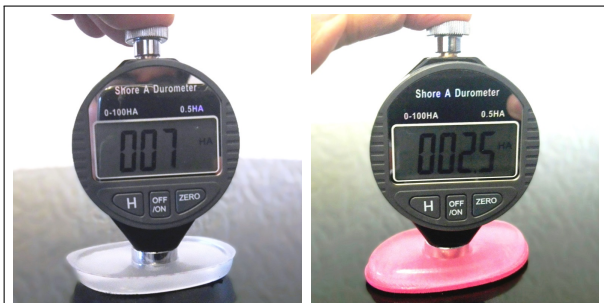
(a) Shore A reading for trans- (b) Shore A reading for silicone with pink cushion. parent silicone sponge.
