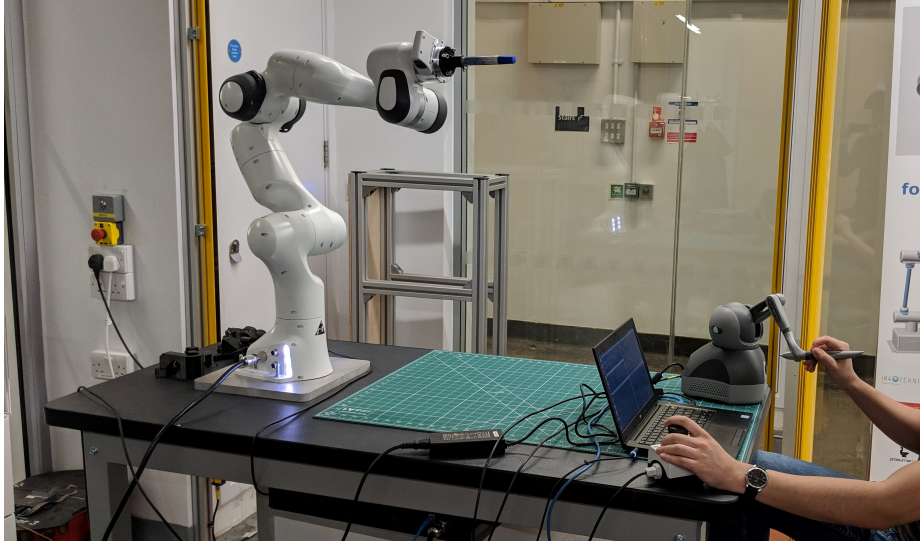
Fig. 2. The experimental setup: slave PC, master and slave robots
