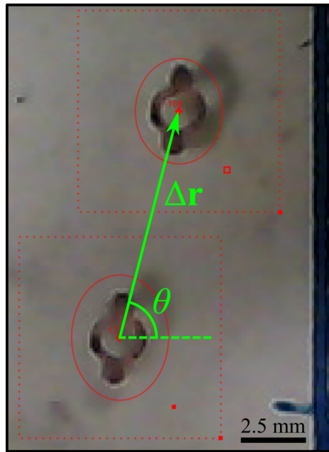
Fig. 3.6 Visualisation of the particle tracking software, showing the position vector, \Delta\mathbf{r} , and angle \theta between two frames of the video. The long axis of the shown swimmer is 3.6 mm.
