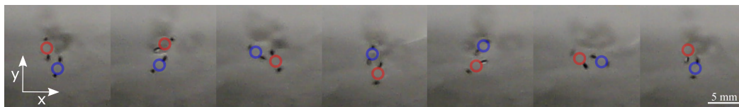
Fig. 7.1 Sequence of images showing the motion of two PDMS two-ferromagnetic particle swimmers (3.6 mm). The coloured rings are overlaid to distinguish between the two swimmers. The magnetic field applied has a strength of 2.5 mT and frequency of 90 Hz.
