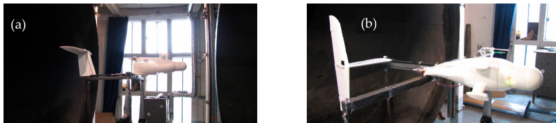
Figure 6. OVLI-TA during the wind tunnel test: (a) angle of attack testing; and (b) angle of sideslip testing [19].
