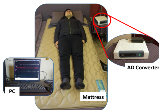
Figure 1. The micro-movement sensitive mattress based BCG signal acquisition system (RS-611).
