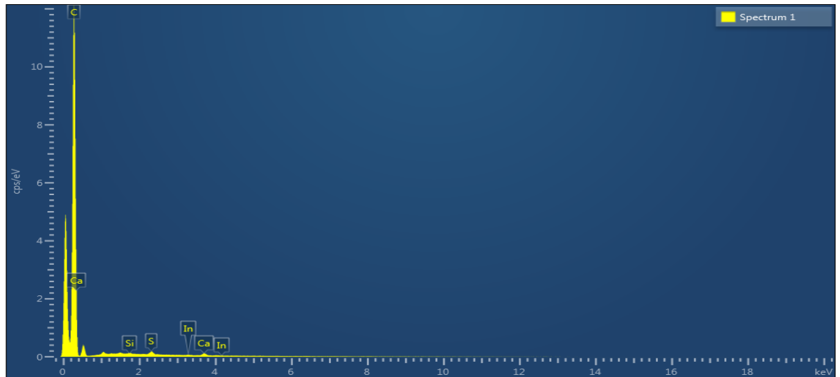
Figure 5.3: Spectrum of the materials detected in the tested sample of conductive paper (Graph counts per second per electron-volt (cps/eV) vs KeV).
