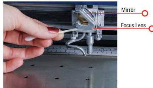
Figure 4.5: Representation of cleaning the optics.
