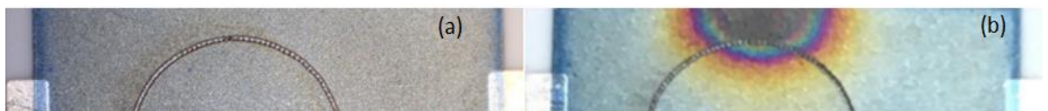
Figure 7.8: (a) Thin film resistor trimmed with the elliptical cut before application of power, (b) the resistor after application of higher power value.
