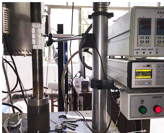
Fig. 10. Testing approach of flexure amplification mechanism
