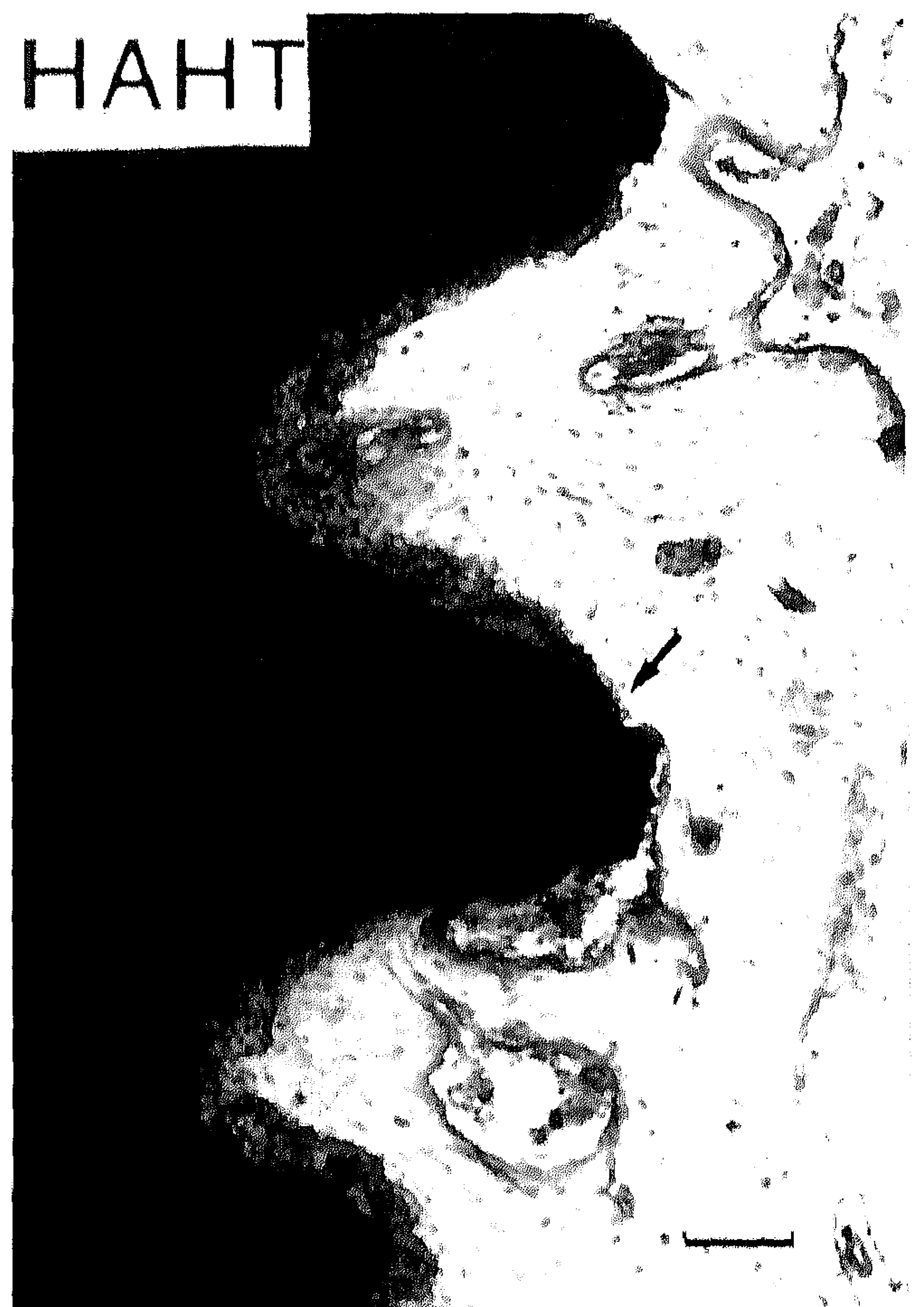
Figure 6. Light micrograph of HAHT-coated implant showing areas of close bone contact with mature bone interrupted by areas of newly formed bone. Even at places where the coating disappeared (arrow), the bone was in close contact with the implant surface. Original magnification: 25 \times , bar = 85 \mu\text{m} .
