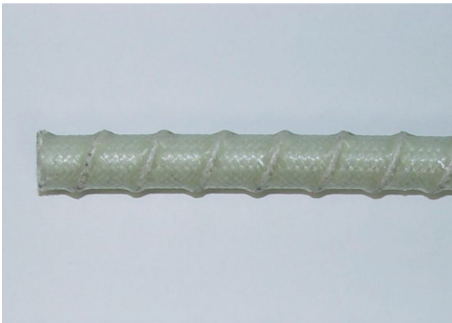
FIGURE 2: KICT GFRP bar [3].
