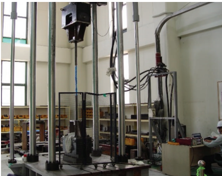
FIGURE 11: Tensile test setup.
