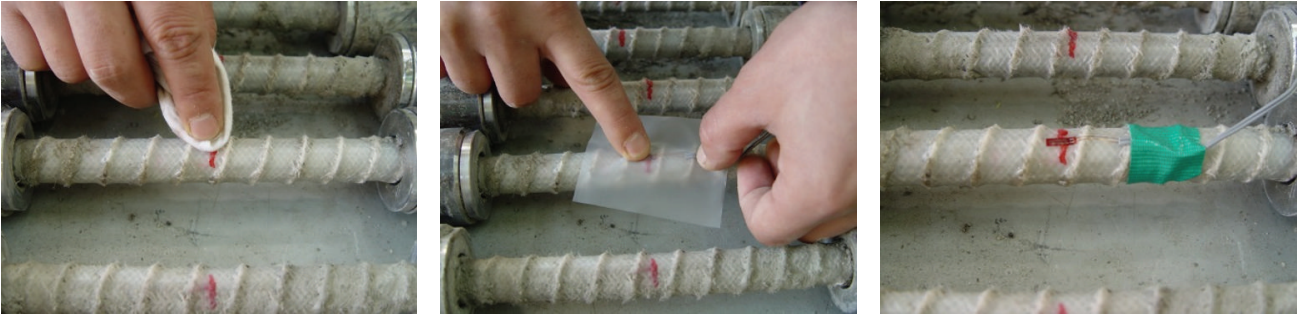
FIGURE 8: The strain gauge attachment.
