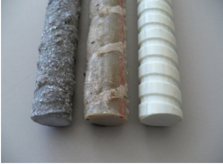
FIGURE 1: Pultrall V-Rod, Aslan 100, and Schöck ComBAR (left to right) [5].
