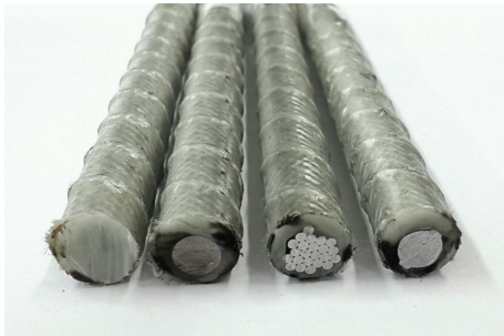
FIGURE 6: The cross section view of FRP Hybrid Bar.
