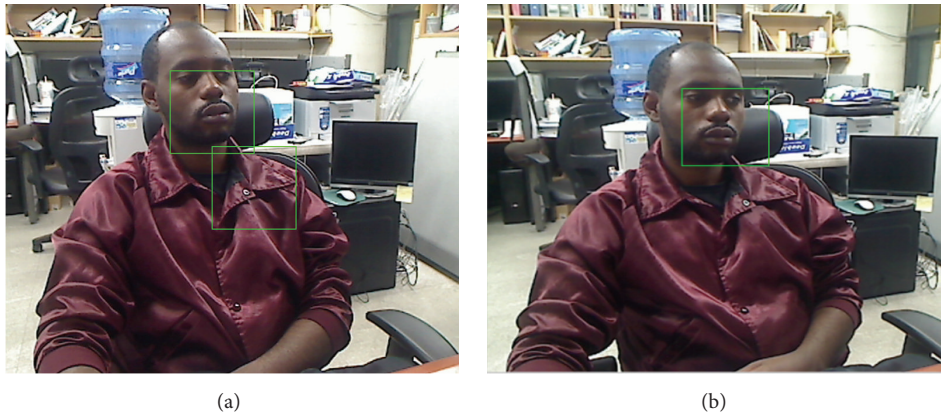
FIGURE 1: Detected faces by the Viola–Jones method (a) and the proposed method (b).
