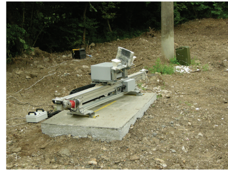
FIGURE 12: Radar installation on the riverbed.
