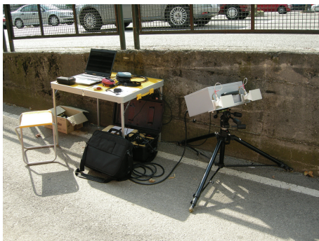
FIGURE 3: Interferometric radar in only-range configuration.
