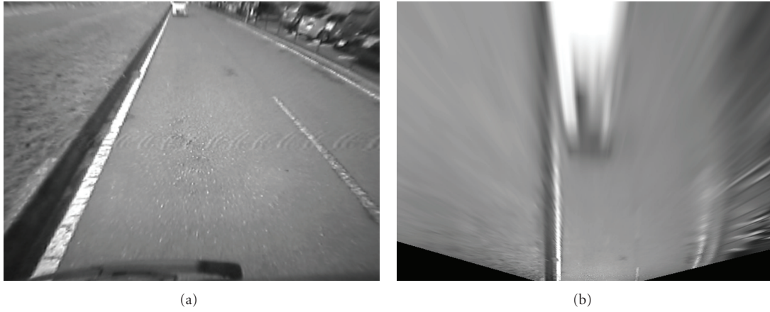
FIGURE 2: Rear camera-view image (a) and top-view image (b).
