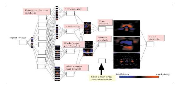
Figure 6. CNN for face detection [33]
