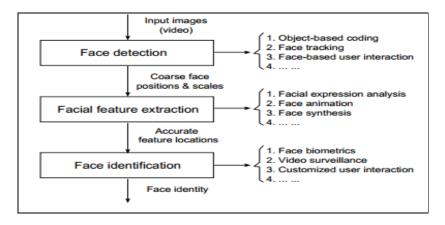
Figure 1. Framework of a face-recognition system [14]
