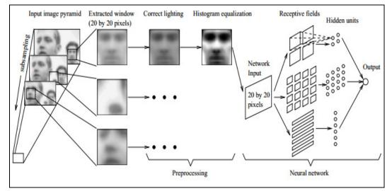
Figure 3. RCNN for face detection [27]
