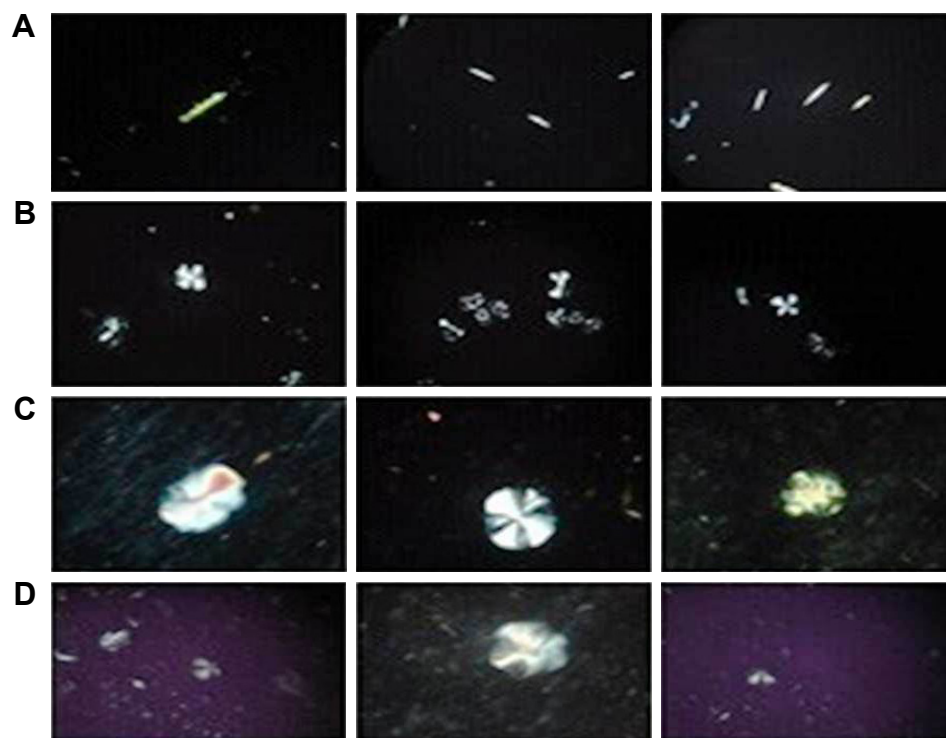
Figure 2 Polarized optical microscopy of AE-LCNPs prepared by thin film hydration method (F6-2) (A), blank LCNPs (B), AE-LCNPs (F6) (C), AE-PEGylated LCNPs (F13) (D). (B–D) Prepared by emulsification technique.
