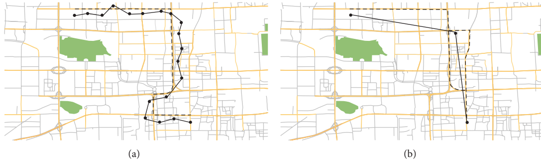
FIGURE 1: A comparison between high-sampling-rate and low-sampling-rate map matching.
