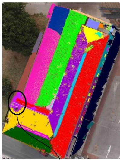
Ground and roof-top object segmented as single element due to radiometric similarity and no 3D information
